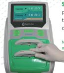
**Step 4.** Close the transfer cassette, pick a channel (A or B) and insert the assembled cassette into the channel.
